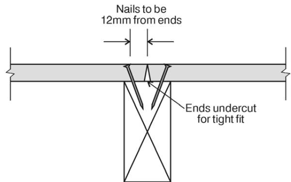
Each board shall be fixed at every joist crossing with two nails as required by Table 5. Alternatively, proprietary fixings may be used in accordance with manufacturer's instructions.
