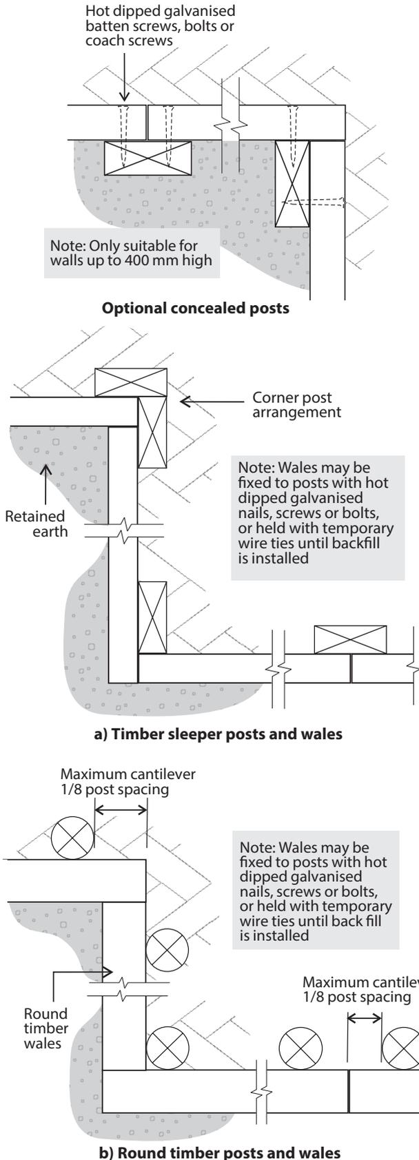
Figure 2 - Positioning Posts at Ends and Corners
