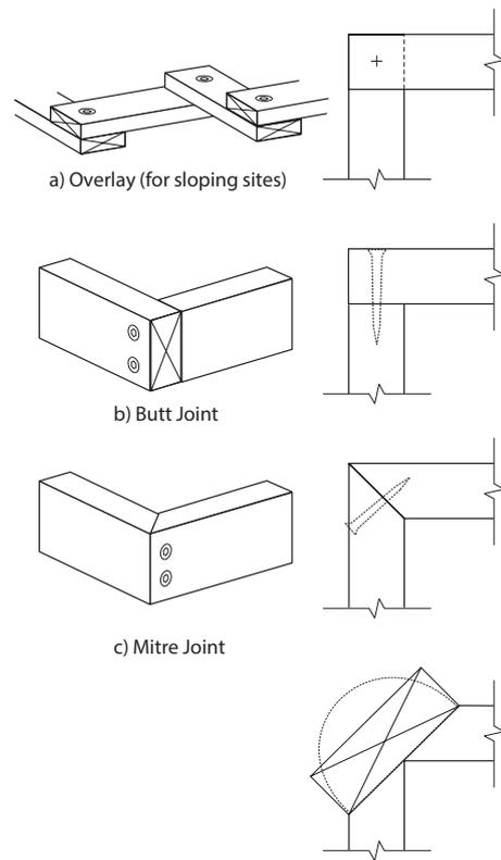
Figure 3 - Typical Methods of Restraining Garden Edges
