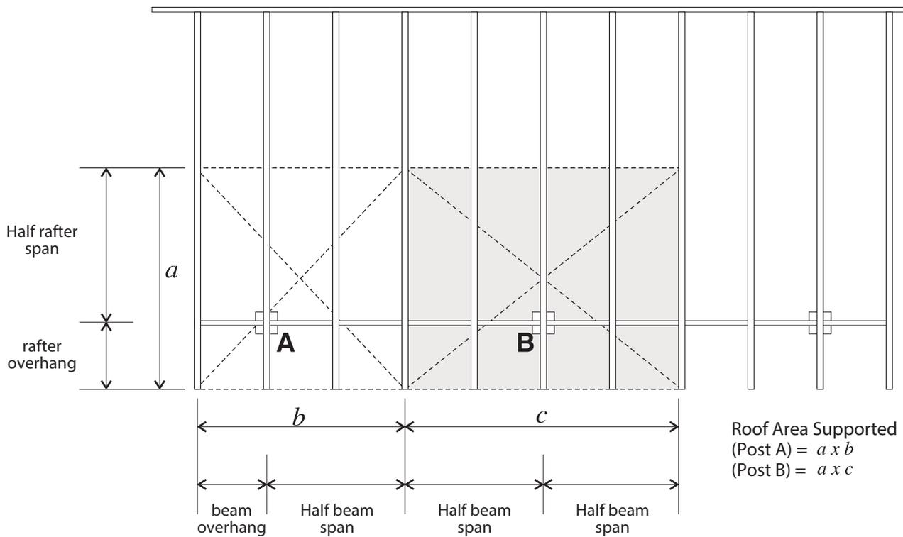
Figure 2 - Roof area supported by posts
