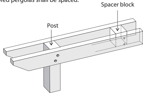
Figure 5 - Multiple beams
