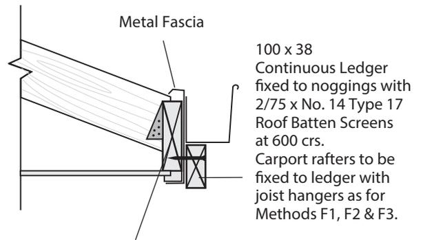
150 x 50 (140 x 45) Nogging fixed between each rafter / truss with 2/75 x 3.15Ø nails or framing anchor each end.
