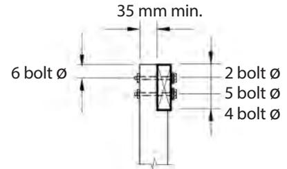
Figure 5 - Example 2 - 1684 typical beam to post detail
